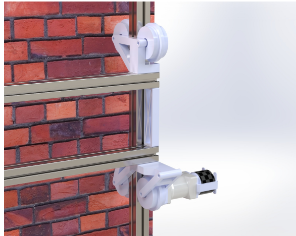
Figure 4.12: Vertical gantry arrangement
